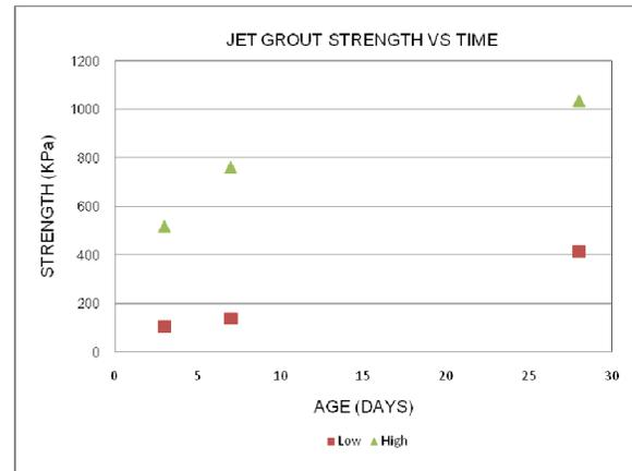
Figure 11 – Jet Grout Strength VS Time
