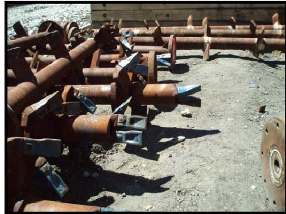
Figure 4 - Detail of Soil Mixing Cutter Heads
