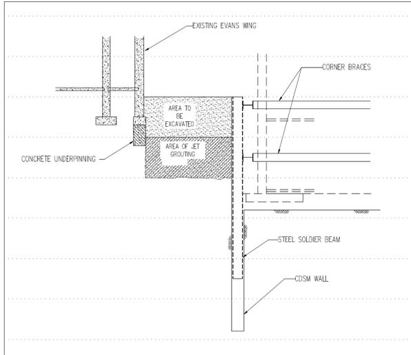
Figure 9 – Section through Jet Grout and Underpinning
