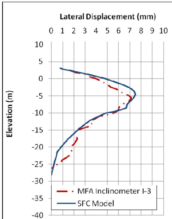
Figure 8 – Comparison of Measured Movements and FEM Model
