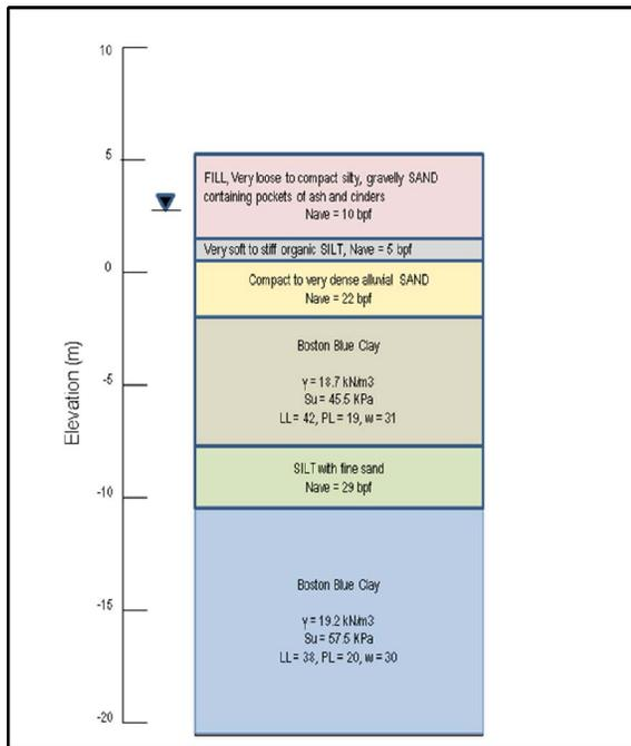
Figure 1 – Typical Soil Profile
