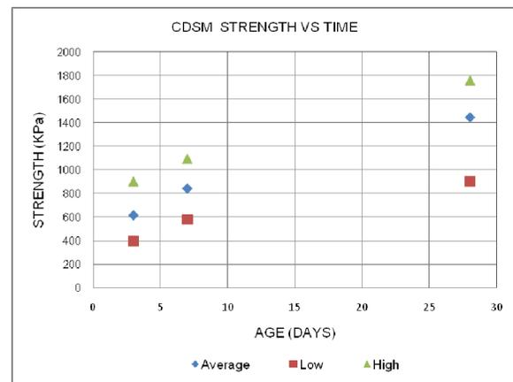
Figure 5 – CDSM Strength vs Time
