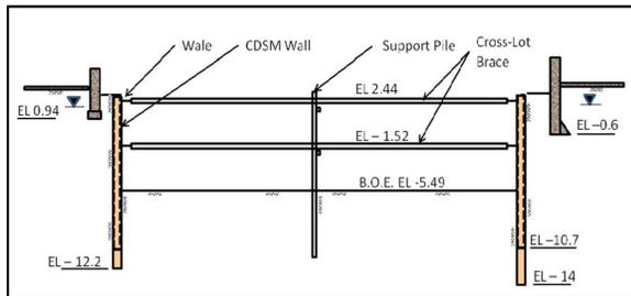
Figure 6 - Section Through ESS at Spine
