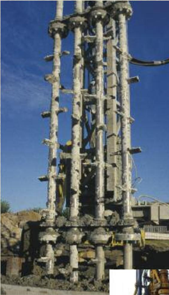
*Schnabel's specialized 4-auger soil mix rig used for the construction of cutoff walls.*
