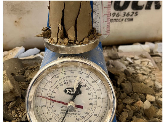
On-site 2x4 cylinder testing
